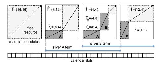
Figure 3: A simple example of resource algebra and sliver allocation. These slivers represent a virtual resource with two dimensions, e.g., virtual machines with specified quantities of memory and CPU power. They are allocated and released from a pool of bounded capacity. Free capacity in the pool is given by vector addition and subtraction as slivers are allocated and released.
