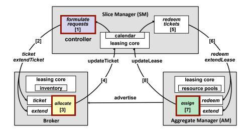
Figure 4: Interacting servers in the ORCA resource control plane. The figure shows the sequence of steps and protocol messages to provision a sliver, passing through policy modules in each server. This figure is adapted from [12].
