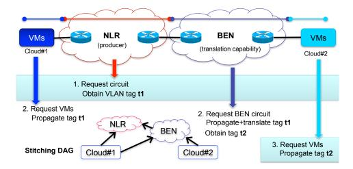
Figure 5: Dependency DAG and stitching workflow for an end-to-end L2 circuit scenario. NLR/Sherpa chooses the VLAN tag at both ends of its circuits, BEN has tag translation capability, and the edge cloud sites can accept tags chosen by the adjacent provider. The connection point descriptions yield a stitching workflow DAG. The controller traverses the DAG to assemble the circuit with a partial order of steps.
