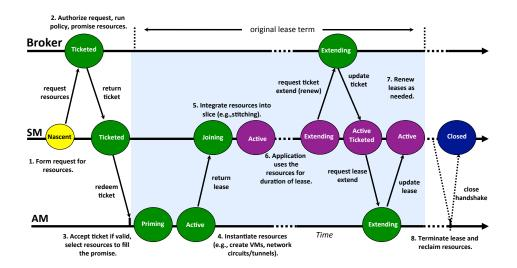
Figure 2: Lease states and transitions. Interacting state machines representing a single ORCA lease at three servers: the SM that requested the resource, the broker that issued the ticket, and the provider (AM) that sets up the slivers, issues the lease, and tears down the resource when the lease expires. Each state machine passes through various intermediate states, triggering policy actions, local provisioning actions, and application launch. This figure is adapted from [15].
