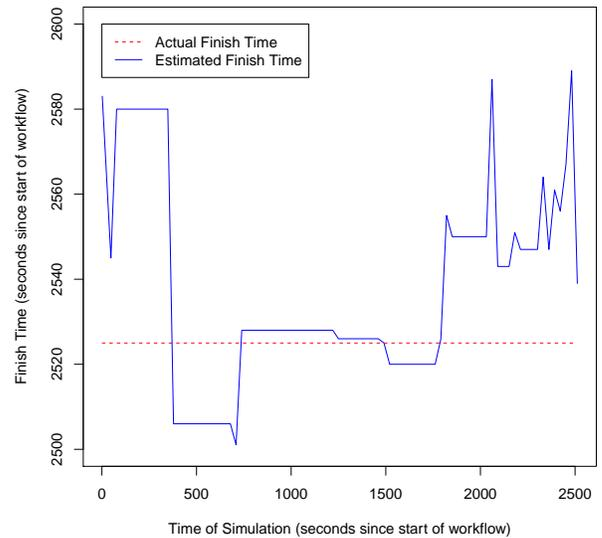
Fig. 5. The majority of estimated workflow finish times predicted by the ShadowQ were within 60 seconds of the actual finish time.
