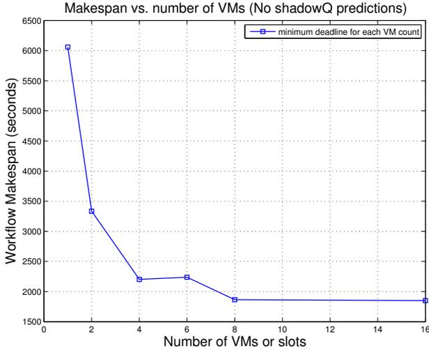
Fig. 7. Workflow makespan vs. number of slots used (no ShadowQ estimates).
